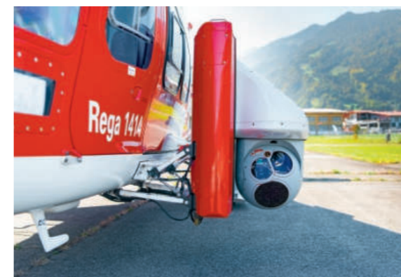
The IR/EOS search system comprises a highly sensitive thermal imaging camera and optical sensors.
