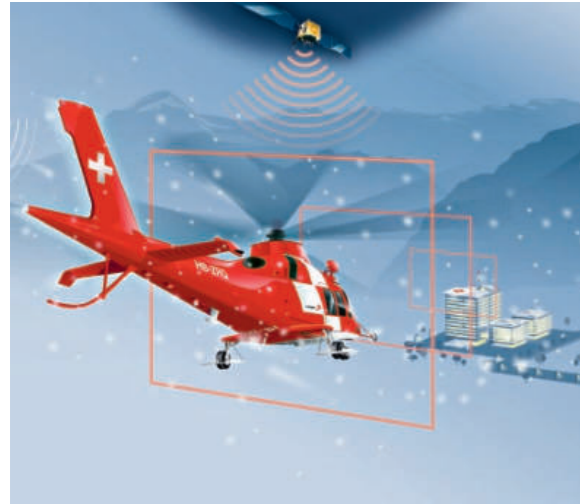
When visibility is poor, the rescue helicopter can follow a flight route stored in the on-board computer.
