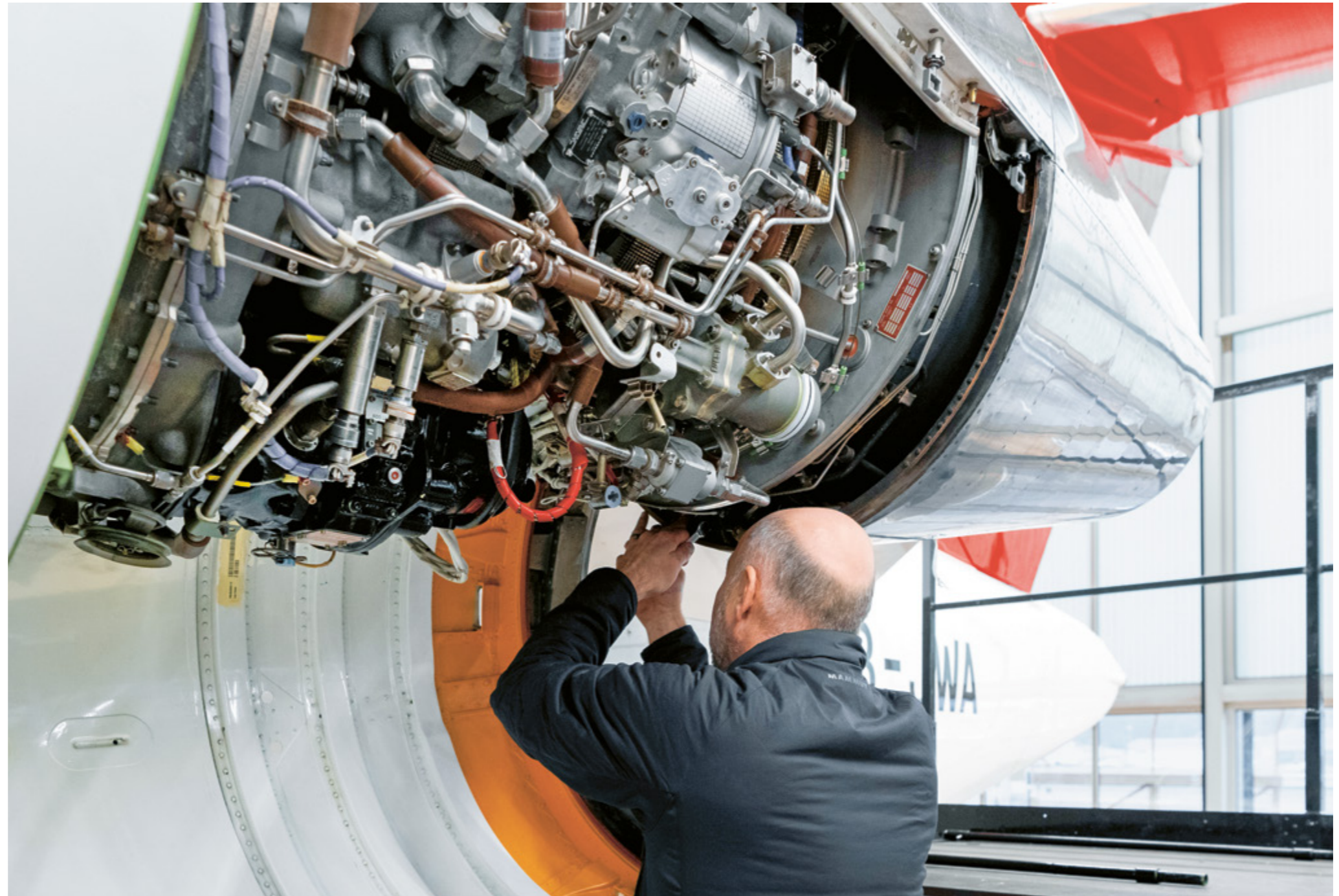
Checking, repairing and maintaining according to the specifications: every six months, the jet mechanics devote themselves to the engine of the ambulance jet.
