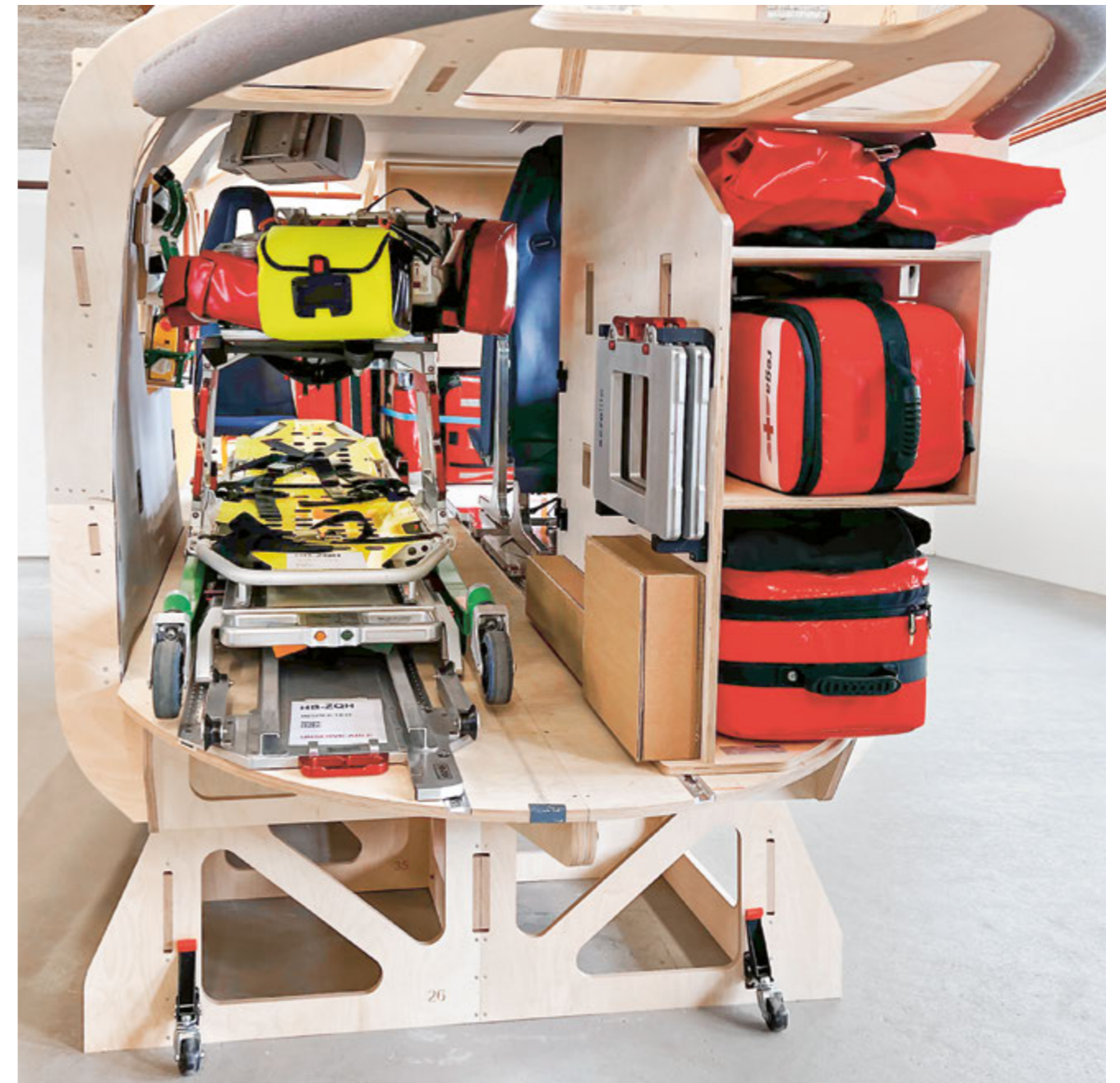
A full-scale wooden model was built to enable adjustments to be made in the cabin.
