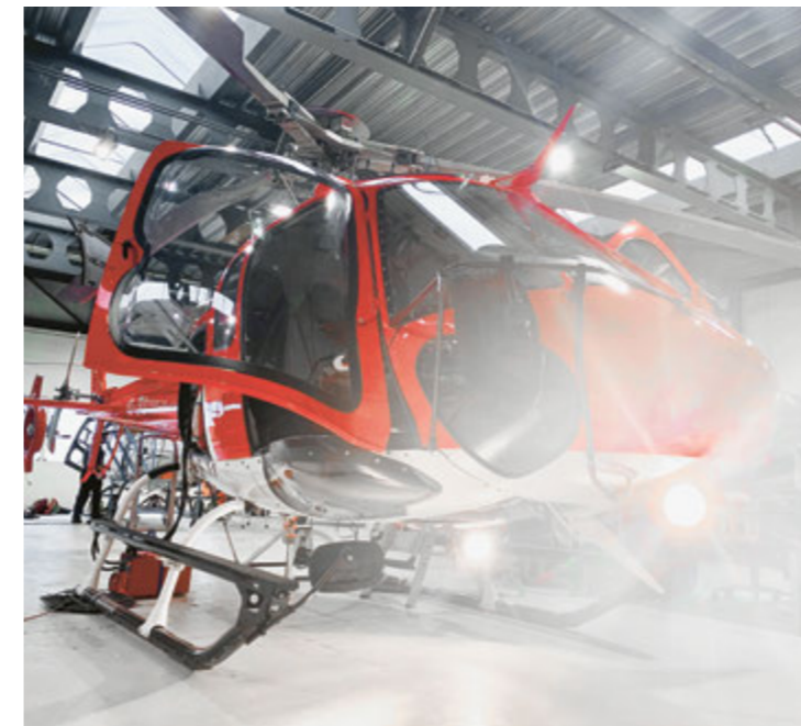
The training helicopter has been fitted not only with an adapted cockpit, but also a new searchlight.
