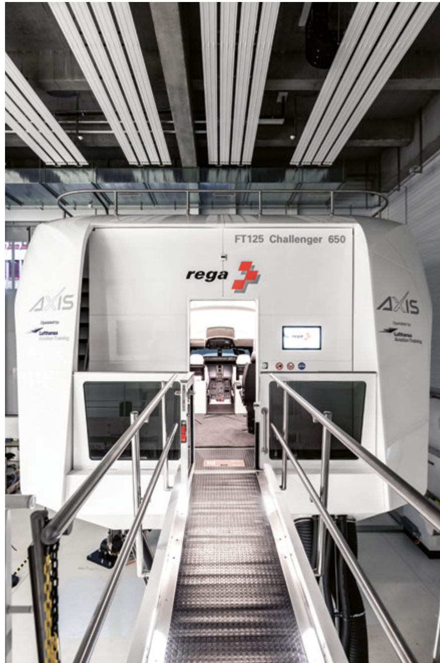
The two simulators (here the jet simulator), which were specially developed for Rega, are standing ready for Rega cockpit crews to train standard situations, as well as emergency procedures that would hardly, if at all, be possible to practise in real life.
