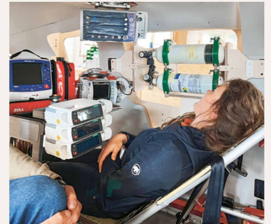
Thanks to the wooden model cabin, the modifications can be extensively tested under the most realistic conditions possible.
