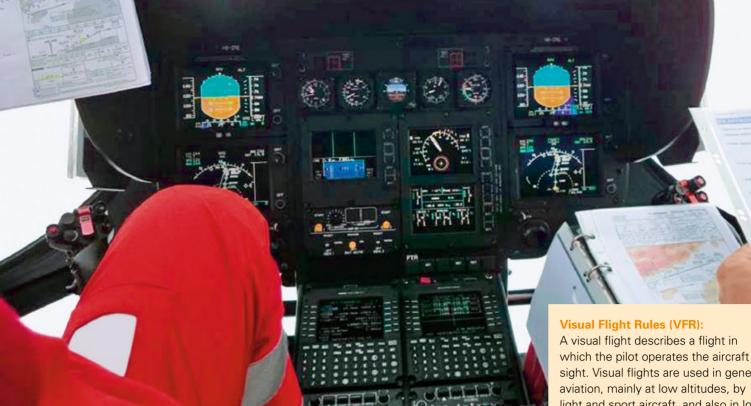
IFR-compatible cockpit: in 2014, all of Rega's Da Vinci helicopters will be equipped for instrument flights.
